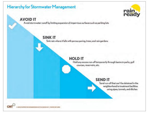
FIGURE DO-2: Hierarchy for Stormwater Management Four main factors contribute to flooding in Dolton:
