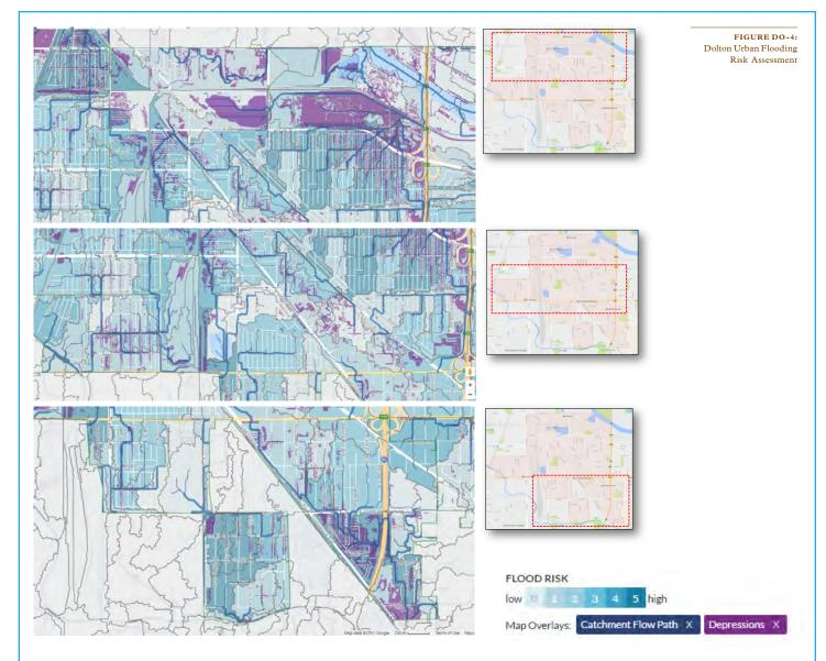
These overland flow path and depression area maps show where stormwater is likely to flow and accumulate, or pool, in Dolton. These maps are based on high-resolution digital elevation models (DEMs) derived from Light Detection and Ranging (LiDAR) technology.
