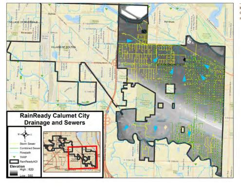
FIGURE CC-3: Calumet City Drainage and Sewers
