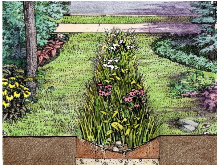
Figure 5. A bioswale uses plants and soil to capture, treat, and move rain from one location to another.
