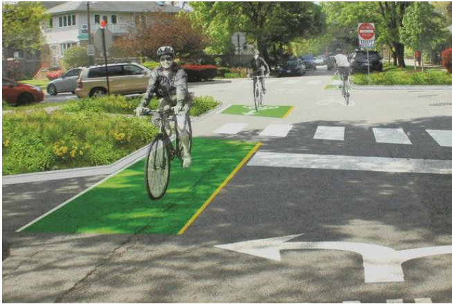
Figure 11. Proposed Manor Greenway, with a traffic diverter, curb extension, and pavement markings. Image Credit: Chicago Dept. of Transportation
